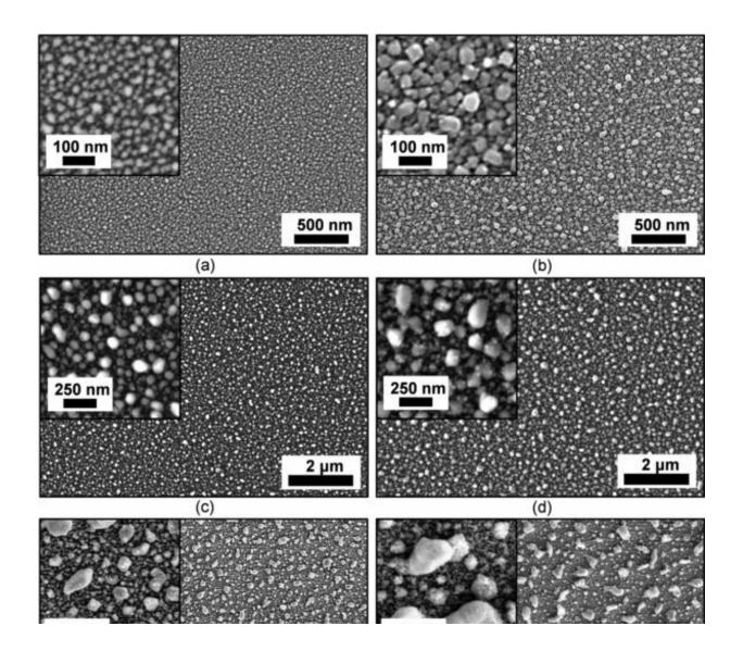
DIC with different patterns. Using this patterning technique, the size of the speckles can be easily manipulated, resulting in a pattern scalable from a few
