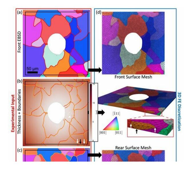
The front and back of a very thin sample. Left experimental measurements of the microstructure, right the numerical "mesh" (discretization of elements) in 3D, with a front view above and a back view below. Credit: Eindhoven University of Technology
