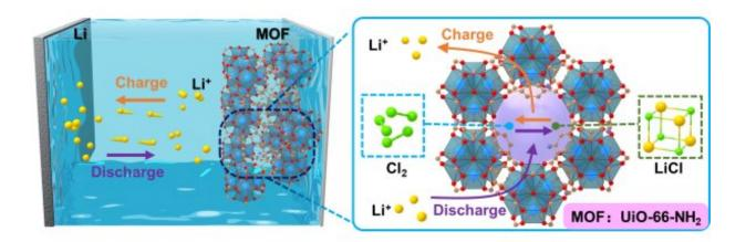
The schematic diagram of the reaction mechanism of Li-Cl<sub>2</sub>@MOF(UiO-66-NH<sub>2</sub>) batteries. Credit: Xu Yan et al
