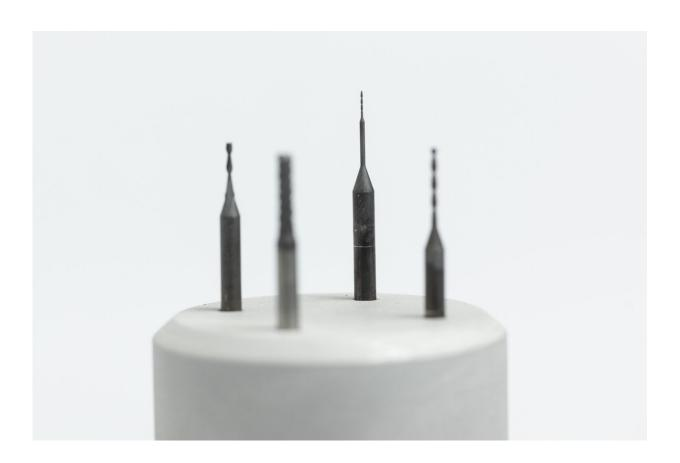
Tools coated with CVD diamond. Credit: Fraunhofer IST
