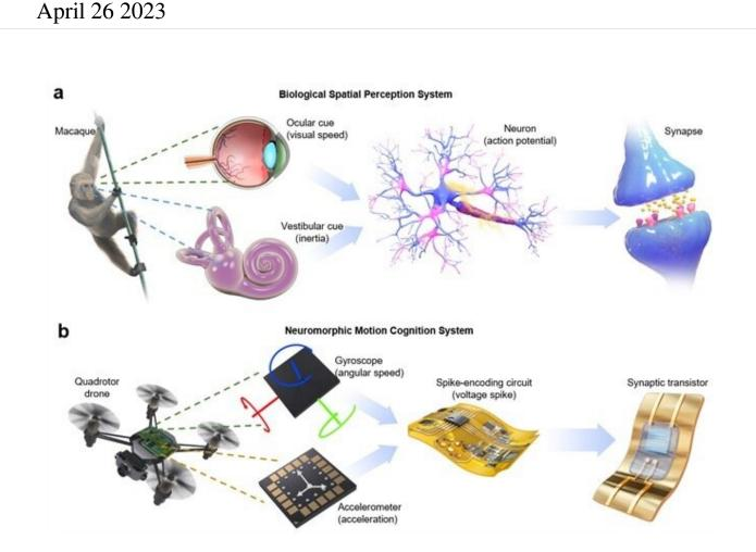
a. Mammalian's ocular/vestibular cross-modal motion sensory system; b. neuromorphic motion perception system based on flexible synaptic transistors. Credit: *Nature Communications* (2023). DOI: 10.1038/s41467-023-36935-w
