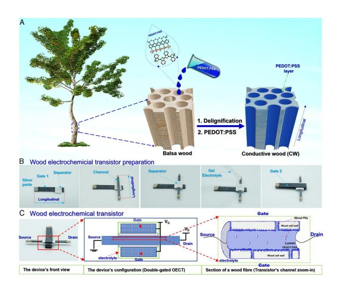
The schematic diagrams of (A) conductive wood preparation and (B) the wood electrochemical transistor fabrication processes. (C) From Left to Right: Front view photograph of a WECT, front view of the WECT configuration, and section of a wood fiber (conceptual view of transistor's channel zoom-in) showing PEDOT:PSS-coated cell wall and electrolyte-transporting lumen.
