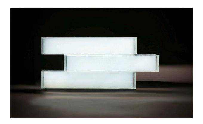
Front view of translucent glass-brick prototypes with transparent side spacers and diffusive light effect. Credit: *Journal of Building Engineering* (2022). DOI: 10.1016/j.jobe.2022.105600
