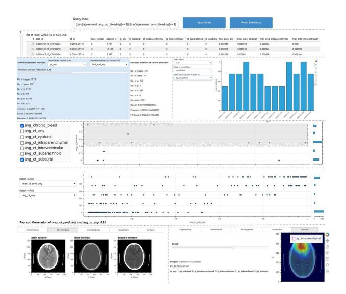
The ScrutinAI tool is used to detect errors in AI models or training data and to analyze the causes. In this example, an AI model for detecting abnormalities and diseases in CT images is being studied. Credit: Fraunhofer IAIS
