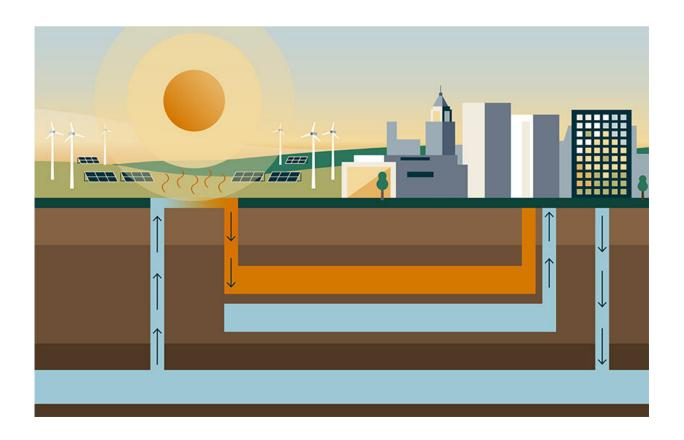
Aquifer thermal energy storage (ATES) uses naturally occurring underground water to store energy that can be used to heat and cool buildings. Credit: Jenny Nuss/Berkeley Lab
