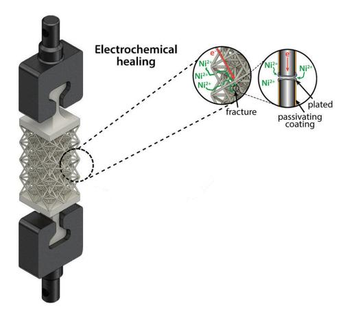
In this 3D rendering of an octet-truss lattice structure, the insets show how nickel ions can easily access the fractured internal strut, where they are reduced to nickel metal during electrochemical healing. A coating enables targeted electrochemical reduction at the fracture site. Credit: Zakaria Hsain
