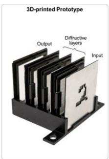
Illustration of an AI-designed unidirectional imager with image formation in only one direction and is capable of maintaining its functionality over a broad spectrum of wavelengths, independent of the light polarization. Credit: Ozcan Lab @ UCLA
