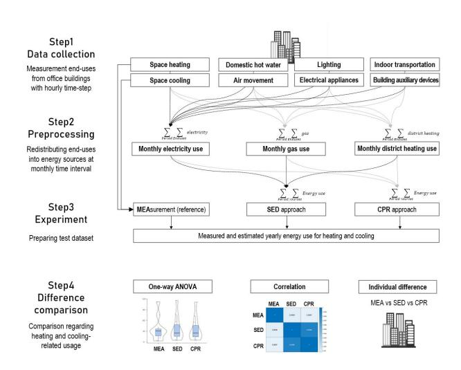
Research flowchart on the disaggregation performance comparison for heating and cooling energy use. It consists of four steps as follows. Credit: Korea Institute of Civil Engineering and Building Technology
