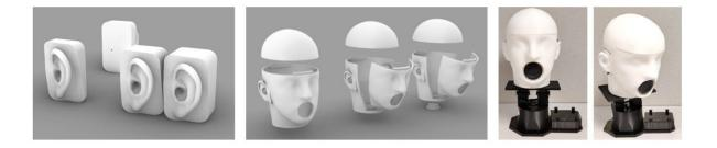
The head simulators are 3D-printed into components and assembled, enabling customization at low cost. Credit: Augmented Listening Laboratory at the University of Illinois Urbana-Champaign
