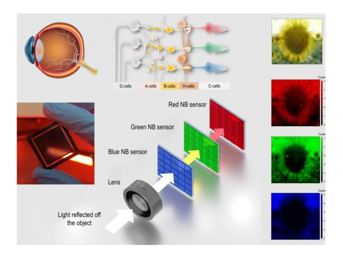
Scientists created a new sensor array from narrowband perovskite photodetectors, which mimic our cone cells, and connected it to a neuromorphic algorithm, which mimics our neural network, to process the information and produce high-fidelity images. Credit: Kai Wang
