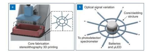
Figure 1. (a) Schematic representation of the core/cladding fabrication using stereolithography 3D printing technique. (b) Representation of the batteries and  $\mu$ LED assembly in the structure. Credit: Compuscript Ltd
