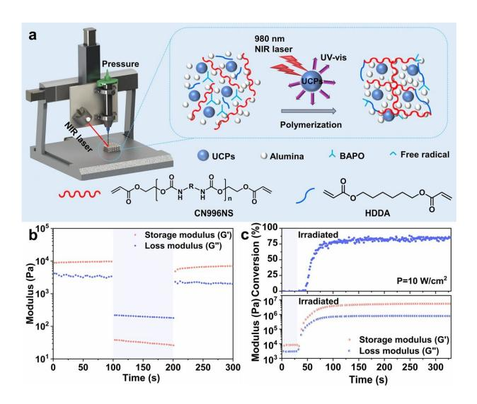
Performance of photosensitive ceramic slurry. **a** Schematic representation of NIR-assisted direct ink writing. **b** Three intervals thixotropic test showing the elastic recovery of the alumina slurry at a frequency of 1 Hz. **c** NIR-induced photopolymerization of slurry was monitored by real-time FTIR rheological analysis. The upper figure showed the double bond conversion as a function of
