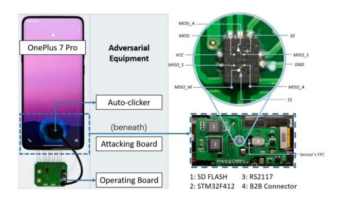
Example of implementing automatic fingerprint bruteforce attack, which uses a suppressible attacking board, a hardware auto-clicker, and an optional operating board. Credit: *arXiv* (2023). DOI: 10.48550/arxiv.2305.10791
