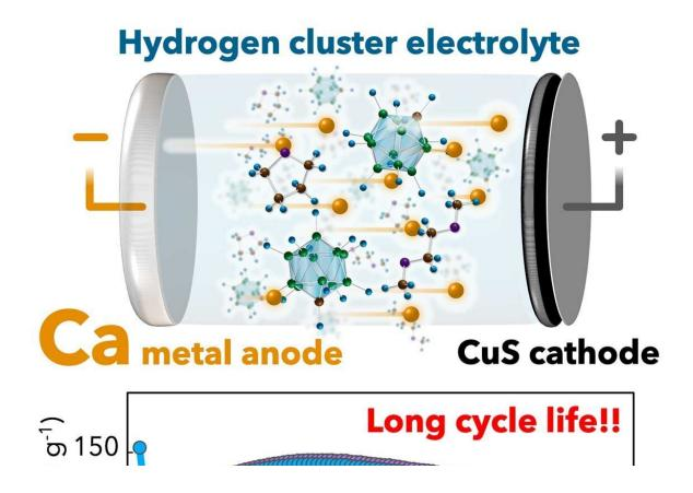
Schematic of a prototype Ca metal battery. The battery comprises a Ca<sup>2+</sup> storing positive electrode containing the CuS cathode and Ca metal anode with a hydrogen cluster electrolyte. Cycling performance of the Ca-CuS battery. Credit: Kazuaki Kisu
