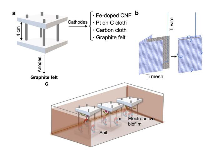
A. Design and electrode materials of the four SMFCs tested in this study. B. Cathode assembly. C. Experimental set-up. Credit: *Environmental Science and Ecotechnology* (2023). DOI: 10.1016/j.ese.2023.100276
