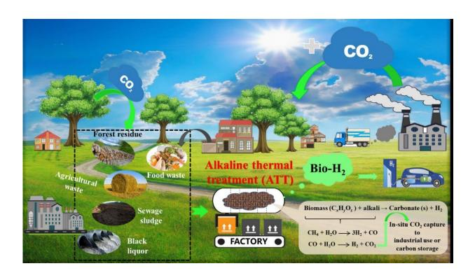
The process of hydrogen production with carbon storage by alkaline thermal treatment of biomass. Credit: the authors
