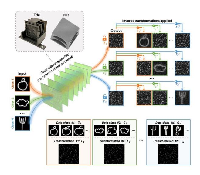
Data class-specific image encryption using a diffractive optical network. The image information is encrypted by the diffractive network in a class-specific manner, which can be retrieved at the output only by applying the correct decryption key (i.e., the inverse transformation). Data from different object
