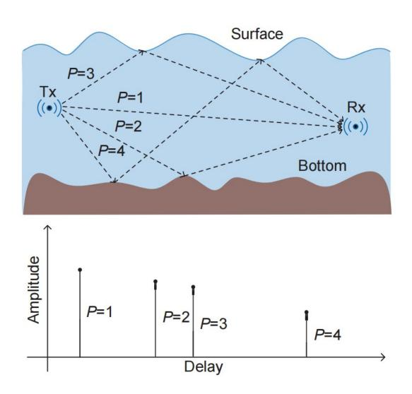
Multipath propagation results in a single signal being received (Rx) through different paths (P=1, P=2, P=3, P=4) and with different delays (lower diagram). This type of interference is modeled in channel estimation to more effectively denoise offshore transmissions. Credit: *Intelligent and Converged Networks*,
