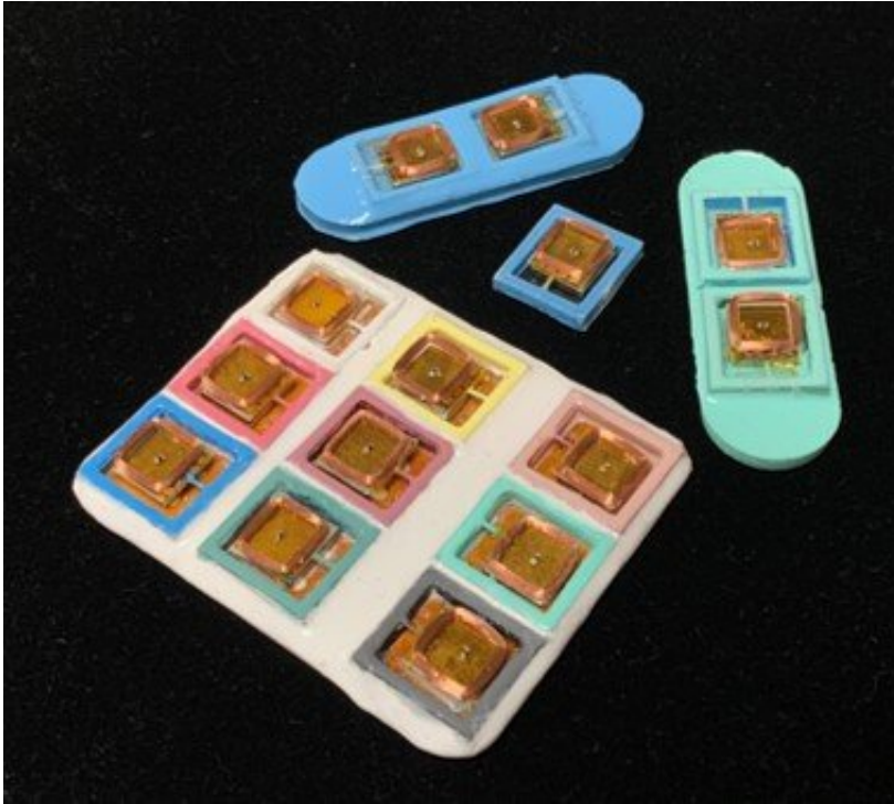
Photos of olfactory interfaces with 1, 2 and 9 odor generators. Credit: Xinge Yu
