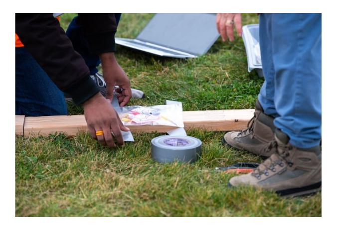
Small samples of radiological sources commonly surveyed during decommissioning—cobalt-60 (Co-60), cesium-137 (Cs-137), and americium-241 (Am-241)—were duct-taped to 2 × 4 boards to create a test track for the drone- and handcart-mounted radiological detectors. The path included an area for measuring background radiation. Credit: Andrea Starr, Pacific Northwest National Laborator
