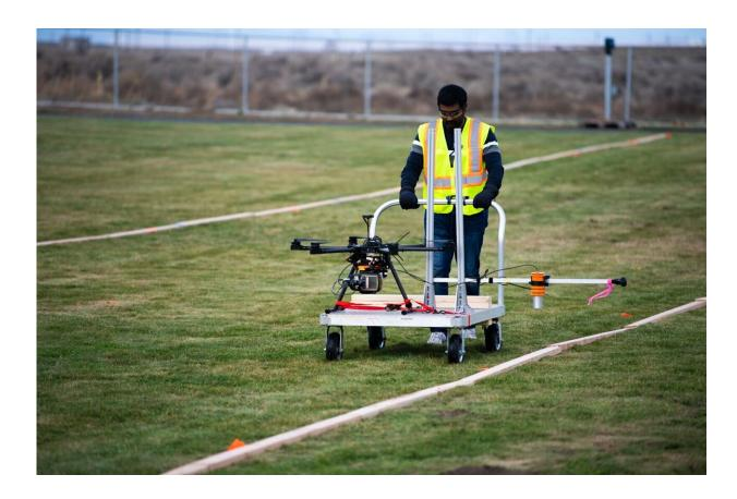
Researcher Harish Reddy Gadey walks a test path as a human surveyor, using a rolling cart to collect radiological data for comparison to the data collected by the same survey devices attached to a flying drone. Credit: Graham Bourque, Pacific Northwest National Laboratory
