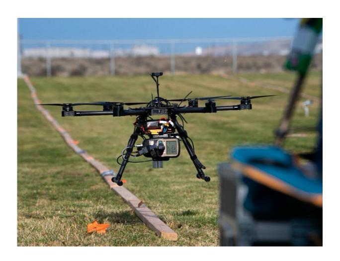
During a study conducted for the U.S. Nuclear Regulatory Commission, PNNL researchers made sure that the drone flew slowly while maintaining an altitude of approximately one foot over the ground for accurate radiological measurements. Credit: Graham Bourque, Pacific Northwest National Laboratory
