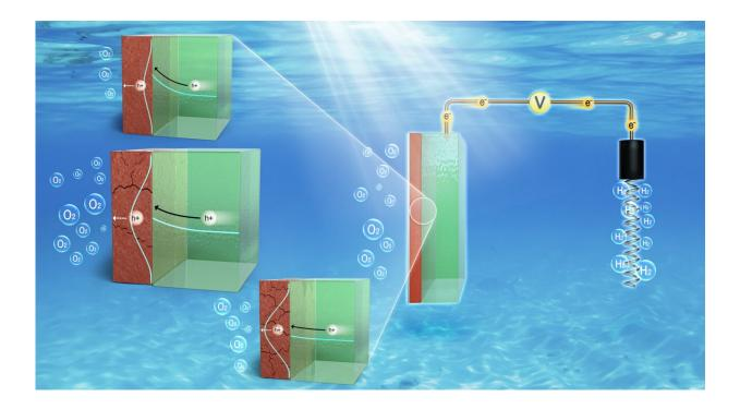
For the efficient PEC water splitting, it is crucial to balance two factors by systematically controlling the defect density in  $TiO_x$  passivation layer of n-Si photoanode, which are (1) accessible density of state for carrier transportation in forbidden gap and (2) favorable interface energetics. Credit: Korea Research Institute of Standards and Science (KRISS)
