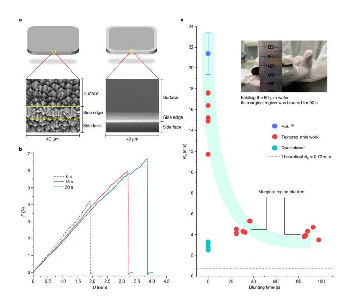
Foldable wafers a, SEM images of a textured c-Si wafer. The sharp pyramids in the marginal region were efficiently removed by an acid solution. b, Load–vertical displacement (F–D) curves of 140-µm textured c-Si wafers, in
