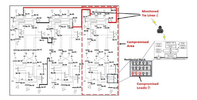
Adapted IEEE RTS-96 bus system and its smart meter components. Credit: *IEEE Access* (2023). DOI: 10.1109/ACCESS.2023.3266249
