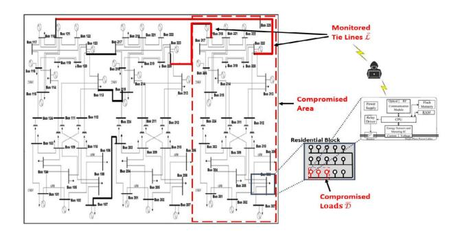
Adapted IEEE RTS-96 bus system and its smart meter components. Credit: *IEEE Access* (2023). DOI: 10.1109/ACCESS.2023.3266249
