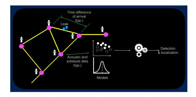
An overview of the methodology utilized for leak identification consisting of collecting acoustic data, extracting relevant features, and employing advanced machine learning and probabilistic models for leak detection and localization. Credit: Pranav Agrawal
