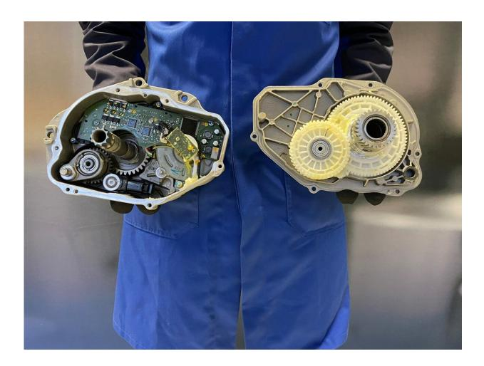
The failure of a component of an electric bike may result in a total loss. In a study, researchers at Fraunhofer IPA have demonstrated that manufacturing spare parts using additive manufacturing is worthwhile. Credit: Fraunhofer-Gesellschaft
