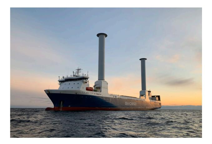
This 2021 photo shows the SC Connector, a freight-hauling vessel owned by the Norwegian company Sea-Cargo, sailing on the North Sea off the southwestern coast of Norway. The ship is equipped with two rotor sails manufactured by Finland-based Norsepower. The 38-yard-high (35-meter-high) rotors spin in the wind and help propel the vessel. It's an example of new technologies helping the shipping industry reduce its greenhouse gas emissions. (Artur Sylwestrzak/Sea-Cargo via AP).
