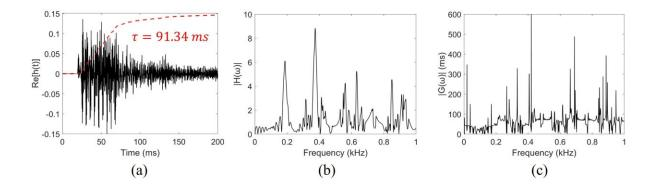
Fig. 2 Calculations of the full-wave channel function, covering the (a) timedomain impulse, (b) amplitude-frequency and (c) group delay responses. Credit: IACAS
