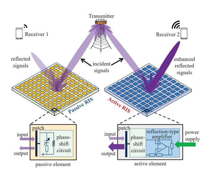
Comparison between the conventional passive RISs and the novel active RISs, where the active RIS is additionally integrated with reflection-type amplifiers to overcome the "multiplicative fading" effect. Credit: Tsinghua Science and
