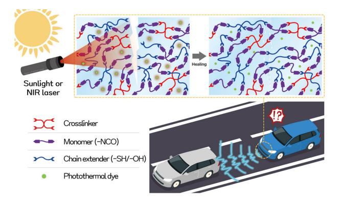
Self-healing mechanism of lens material for self-driving cars using based on a dynamic polymer network and photothermal dye. Credit: Korea Research Institute of Chemical Technology (KRICT)
