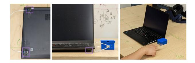
A sensing system called SAWSense takes advantage of acoustic waves traveling along the surface of an object to enable touch inputs to devices almost everywhere. Here, a table is used to power a laptop's trackpad. Credit: Interactive Sensing and Computing Lab, University of Michigan
