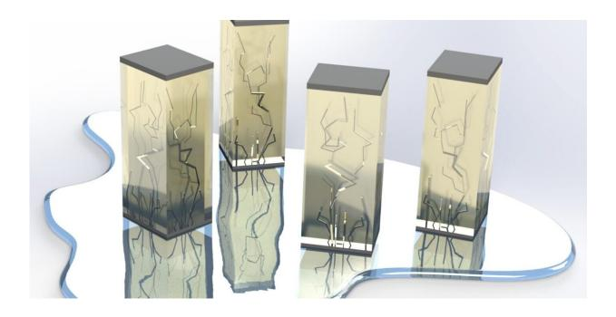
Ceramic solid electrolyte cells (vertical rectangular shapes) with dendrites (the lightning-like dark structures inside the rectangles) growing inside them from the bottom to the top. These solid electrolytes are floating on a liquid (blue puddle) which represents a liquid electrolyte. The reflections of the solid electrolytes in the blue liquid, particularly the dark dendrites, show the similarity in the dendrite initiation process in both the liquid and solid. Credit: Rajeev Gopal/Bai lab
