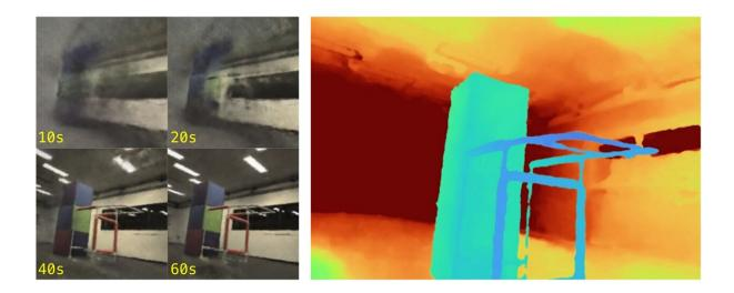
(Left) Renderings from a NeRF that is created using a camera equipped quadrotor and NerfBridge at different times. (Right) Depth reconstruction from the same NeRF showing accurate reconstruction of the scene geometry. Credit: Yu et al
