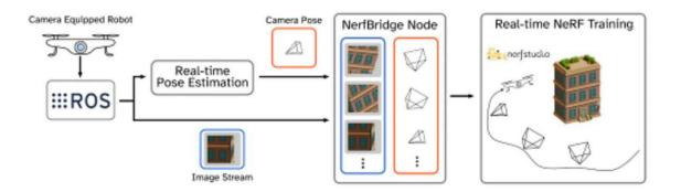
A visualization of how NerfBridge integrates with robot systems and NerfStudio. Images are streamed from the robot, and camera poses are estimated in real time. Posed images are then passed to NerfBridge which in turn inserts them into the training data set for an instance of NerfStudio. Credit: Yu et al
