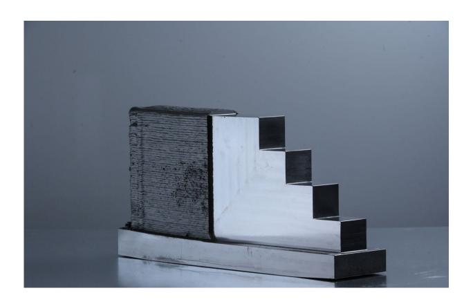
Sample component produced by deposition welding with a mass of around 18 kilograms applied. Credit: LZH
