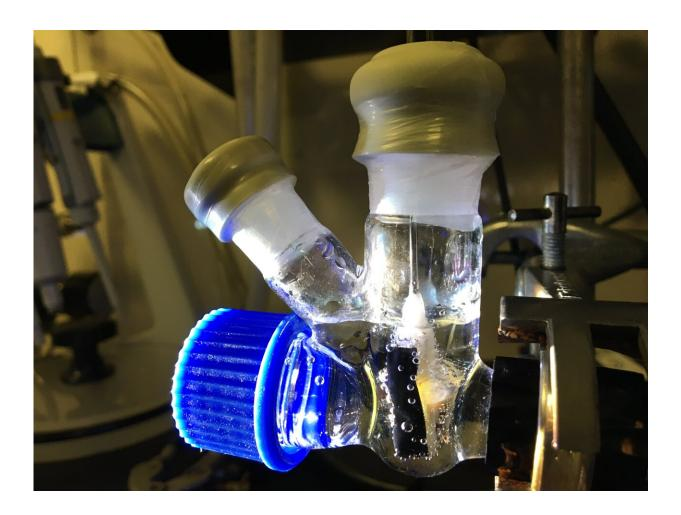
A photoreactor with an artificial leaf working under solar irradiation. Credit: Motiar Rahaman
