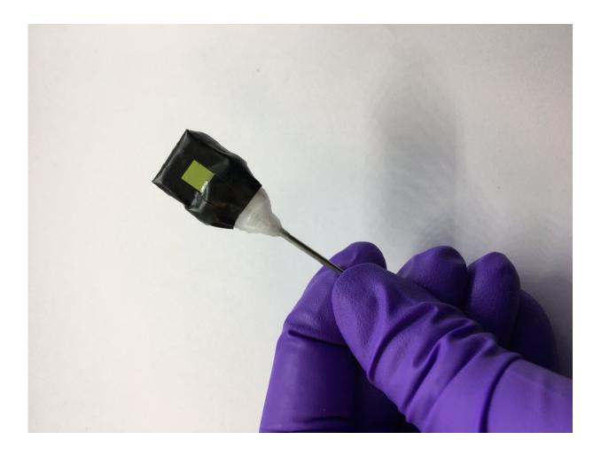
A standalone artificial leaf attached to a metal rod support. The photoanode side (green square) is visible in the photograph. Credit: Motiar Rahaman
