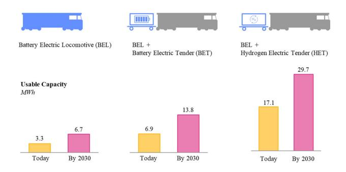
Potential platforms for decarbonization. Current usable capacities are based on commercially available technology, and future capacities are based on known technology advancements by the end of the decade. The calculated energy capacity takes depth of discharge limits and battery life degradation into account. Credit: *Journal of Energy Storage* (2022). DOI: 10.1016/j.est.2022.105813
