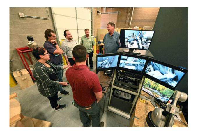
The mobile hot cell can be controlled and monitored from the outside, behind plenty of shielding. Credit: Idaho National Laboratory
