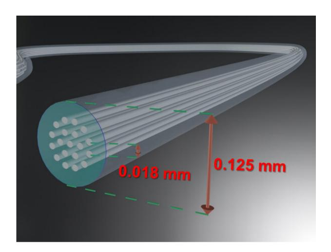
Image of the developed 19-core optical fiber. Credit: National Institute of Information and Communications Technology (NICT) and Sumitomo Electric Industries, Ltd.
