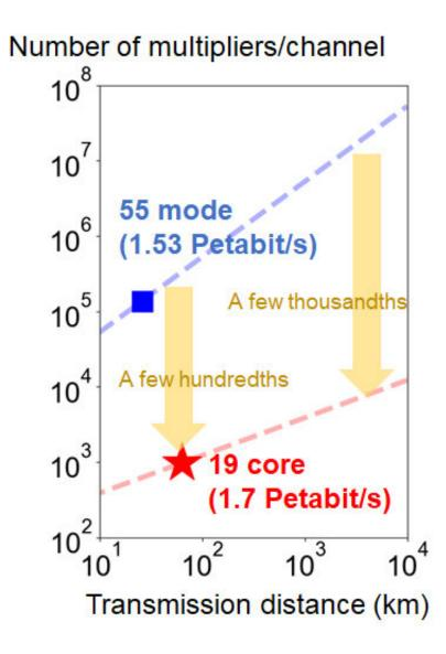
Required number of multipliers per channel in MIMO digital signal processing versus transmission distance. Credit: National Institute of Information and Communications Technology (NICT) and Sumitomo Electric Industries, Ltd.
