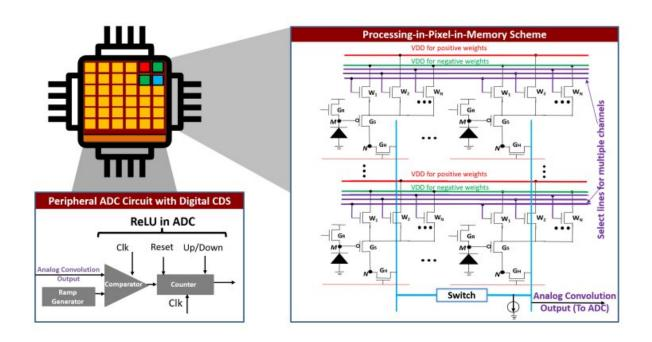
Proposed circuit techniques based on presented P<sup>2</sup>M scheme capable of mapping all computational aspects for the first few layers of a modern CNN layer within CIS pixel arrays. Credit: *arXiv* (2022). DOI: 10.48550/arxiv.2203.04737
