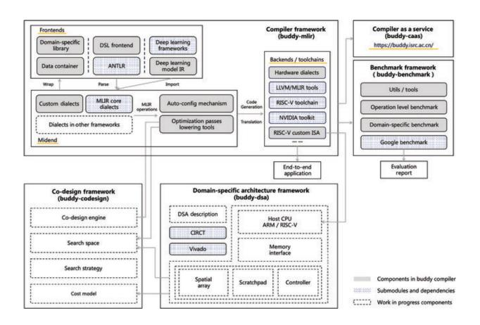
The Buddy Compiler framework, a work in progress, will include a benchmark framework, a domain-specific architecture framework, a co-design module, and a compiler-as-a-service platform in addition to a compiler framework. Credit: Hongbin Zhang et al.
