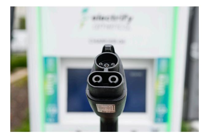
A Combined Charging System (CCS) plug is photographed at an EV charging station in Anaheim, Calif., Friday, June 9, 2023. Currently in the U.S. there mainly are two types of EV charging plugs, Tesla's North American Charging Standard, and CCS1, which is now used by nearly all other automakers but Tesla. Credit: AP Photo/Jae C. Hong
