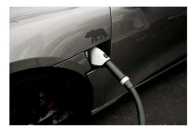
A Combined Charging System (CCS) connector is plugged into an electric vehicle at a charging station in Anaheim, Calif., Friday, June 9, 2023. Currently in the U.S. there mainly are two types of EV charging plugs, Tesla's North American Charging Standard, and CCS1, which is now used by nearly all other automakers but Tesla. Credit: AP Photo/Jae C. Hong
