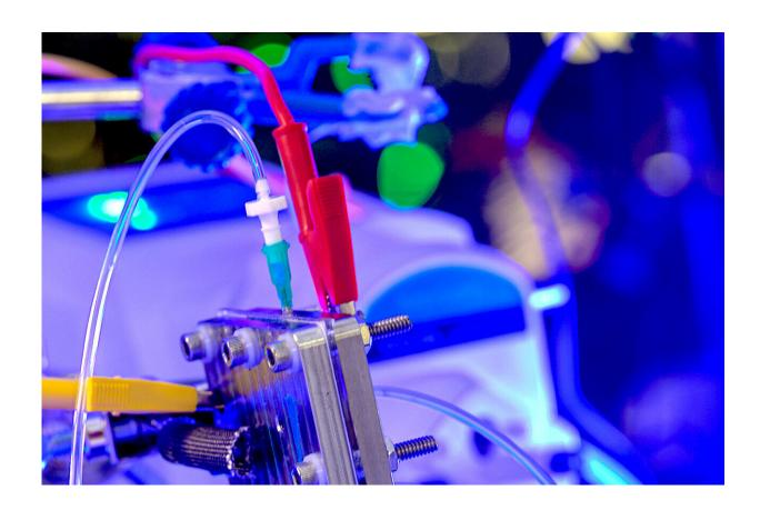
The reactor is made up of a cathode set up to perform oxygen reduction, an oxygen evolution reaction-performing anode and a compact yet porous solid-electrolyte layer that allows efficient ion conduction. Credit: Jeff Fitlow/Rice University
