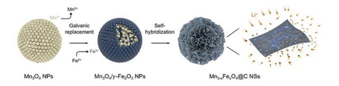
By synthesizing "manganese ferrites" anode material into nanosheets with larger surface area, more lithium ions can be stored, overcoming its theoretical limits.
