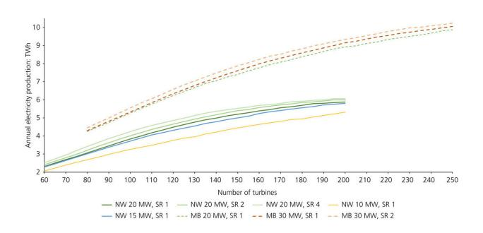
AEP for a Morecambe Bay barrage and North Wales coastal lagoon with various numbers of turbines, generator ratings and SRs. Credit: *Proceedings of the Institution of Civil Engineers - Energy* (2023). DOI: 10.1680/jener.22.00077
