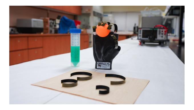
The wooden robotic gripper developed by NUS researchers can spontaneously stretch and bend itself in response to moisture, thermal and light stimulation. It also has good mechanical properties, able to perform complex deformation, wide working temperature range, low manufacturing cost, and is biocompatible. Credit: National University of Singapore
