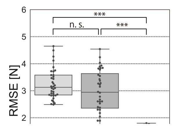
In the comparison of the root mean square errors of the contact force, three conditions were examined: 1) P-N (Pneumatic Force + No Friction
