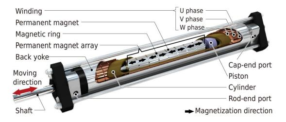
Three-dimensional computer-aided design image of integrated pneumaticelectromagnetic hybrid linear actuator, an example of one realization of the fusion hybrid linear actuator. Note that the part of the model is sectioned. Credit: The University of Electro-Communications
