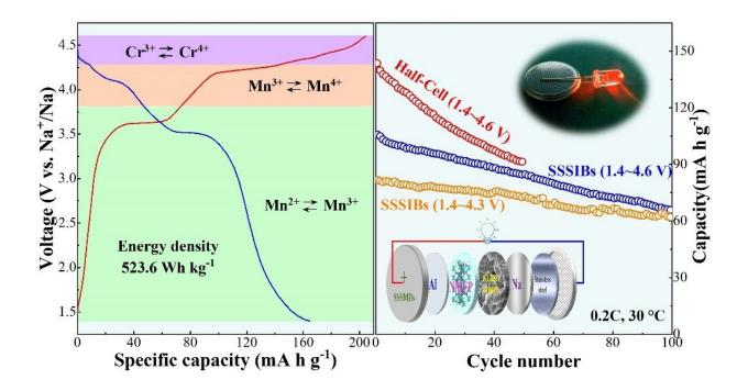
Scientists from Nanjing University of Posts and Telecommunications developed SSSMBs using a high energy Na<sub>4</sub>MnCr(PO<sub>4</sub>)<sub>3</sub> cathode. Credit: Zhongyue Wang, Nanjing University of Posts and Telecommunications
