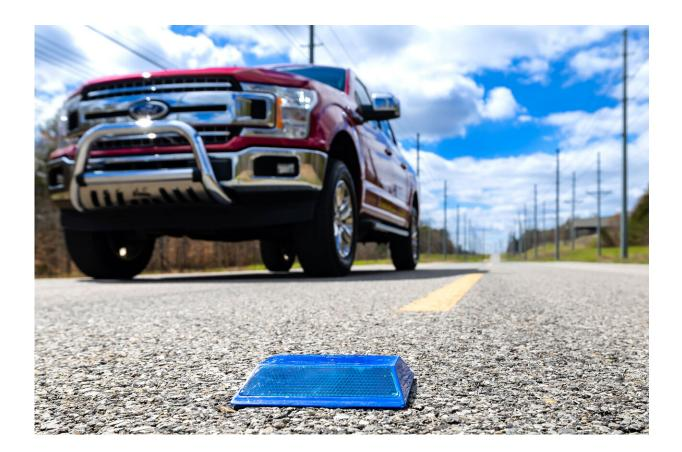
ORNL researchers have enabled standard raised pavement markers to transmit GPS information that helps autonomous driving features function better in remote areas or in bad weather. Credit: Carlos Jones/ORNL, U.S. Dept. of Energy
